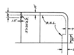
TYPICAL DETAIL FOR BUILDING SETBACK LINE (B.S.L.) AND ANCHOR EASEMENT (3'X20'A.E.)
